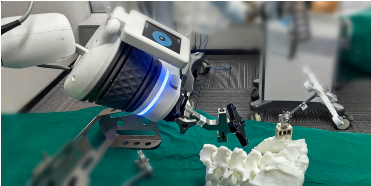
The robotic arm that helps to navigate surgery
